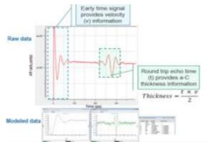
Figure 2. Raw signal and modeling example of measurement on a-C films using PULSE Technology
