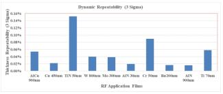
Figure 1. Typical repeatability performance for different stacks of common RF applications
