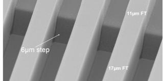
Fig. 6. Photoresist image of RDL over topography
