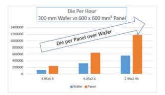
Fig. 8. Productivity increase that can be expected when processing on  $600 \times 600 \text{ mm}^2$  panel over 300mm diameter wafer
