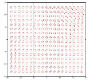
**Fig. 3.** Vector map of die placement offset on a reconstituted panel (Note: Circle radius =  $4\mu m$ )
