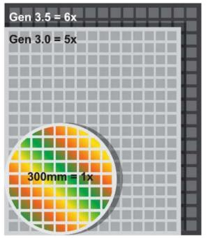
Fig. 1. Comparison of die exposed on 300mm Vs. Panel
