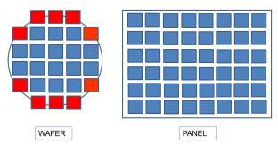
**Fig. 7.** Illustration of partial die exposure on a wafer compared to die exposure on a panel, non-productive areas of die on wafer shown in red
